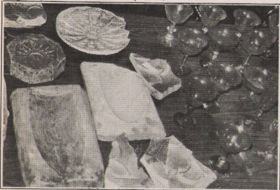
These plaster casts appear to be taken from finished cut glass, to be used as reference points for future designs. At the right are some uncut blanks.
